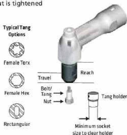
A Bit holds the bolt while the nut is tightened
