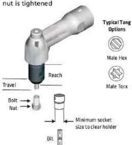
NOTE: The bolt can extend beyond the nut no more than the specified travel distance when tightened.
