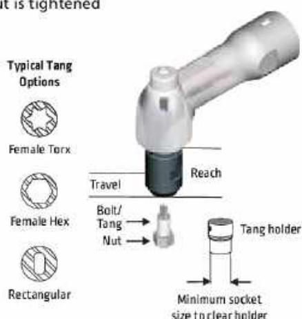
NOTE: The bolt can extend beyond the nut no more than the specified travel distance when tightened.
