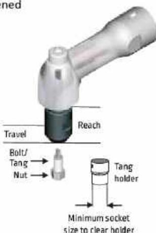
A Bit holds the bolt while the nut is tightened
