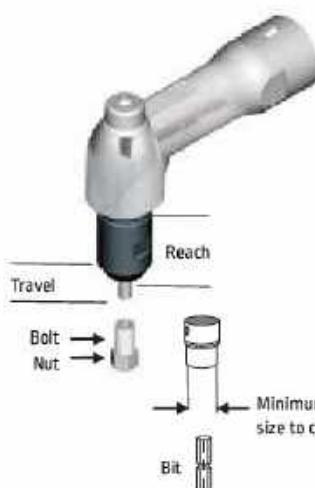
NOTE: The bolt can extend beyond the nut no more than the specified travel distance when tightened.
