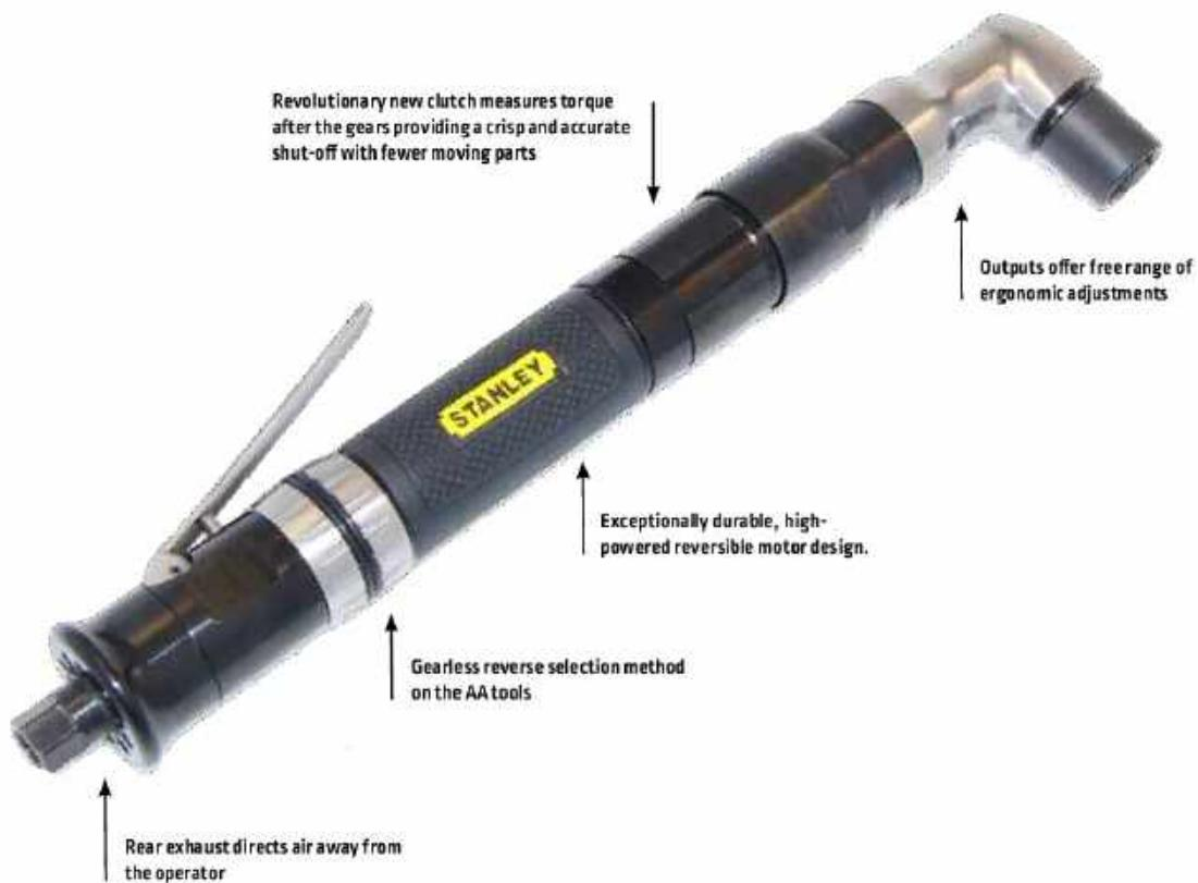
AA Series Pneumatic Tools conform to ISO standards 28927-2 and 15744 for noise and vibration. Actual vibration of AA23 and AA33 series tools is <2.5 m/sec<sup>2</sup>. AA23 series tools' noise was measured at 79 dBA sound pressure levels. AA33 series tools' noise was measured at 85 dBA sound pressure levels. AA33 series tools' noise was measured at 96 dBA sound power level.
